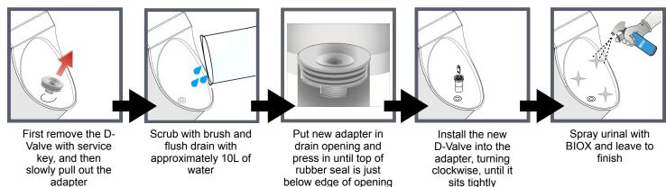
The adapter that the D-Valve sits in needs to be changed on average every 2-3 years depending on usage. The manufacturer recommends using the BIOX microbiological cleaning agent as this does not contain any products that will damage the urinal.
