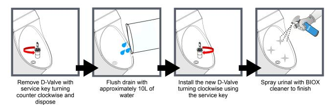
D-Valve needs to be changed on average between 2-4 times a year depending on usage. The manufacturer recommends using the BIOX microbiological cleaning agent as this does not contain any products that will damage the urinal.
